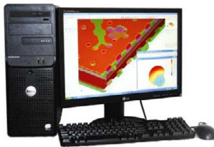
Figure 3.4 An EM simulation workstation with multiple cores or multiple processors. Today, we can easily place four CPUs with 48 cores and 48 VALUs inside one computer.
