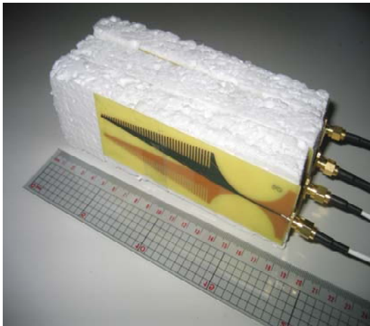
Figure 6.17 Prototype of the UWB antenna array that is used in the experiment.
