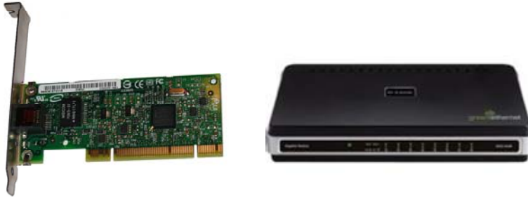
Figure 3.8 Typical Ethernet network card and switch used in the small cluster. (Images from http://en.wikipedia.org .)
