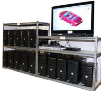
Figure 3.7 High-performance network system allows us to connect the lab/office PCs to form intermediate-sized cluster.
