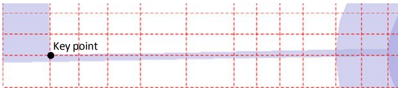
Figure 4.3 Using a key point for a specially shaped structure can significantly reduce the number of unknowns.
