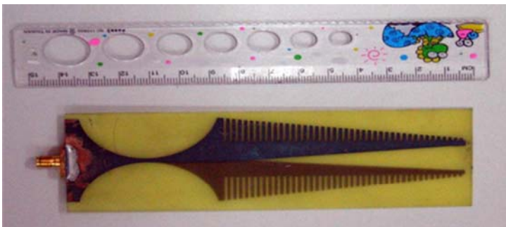
Figure 6.10 Configuration of the comb-shaped antenna element used in the experiment.
