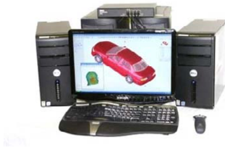
Figure 3.5 A four-port network switch can connect four regular PCs together to form a typical PC cluster. The network cost can be ignored compared to the computer price.
