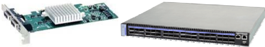
Figure 3.11 InfiniBand network card and switch used in the intermediate-sized or large clusters, and has the fabric and coaxial cards, cables, and switches. (Images from http://en.wikipedia.org .)
