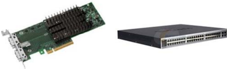
Figure 3.9 The 10-gigabit Ethernet network card and switch used in the intermediate-sized cluster. (Images from http://en.wikipedia.org .)
