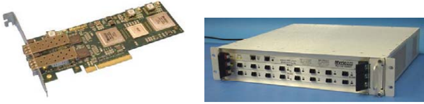
Figure 3.10 Myrinet network card and switch with low latency used in the large cluster with excellent parallel performance. (Images from http://en.wikipedia.org .)
