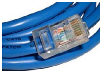
Figure 3.12 A 1-gigabit Ethernet network cable used to connect the two computers directly or from the computers to switch. (Image from http://en.wikipedia.org .)
