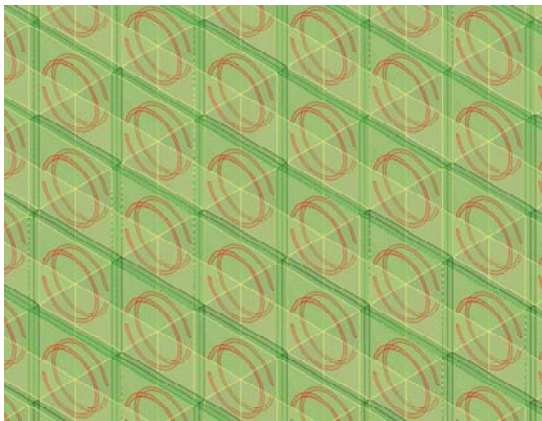
Figure 4.54 Configuration of the periodic structure in the two directions. Each element contains a pair of open PEC rings.
